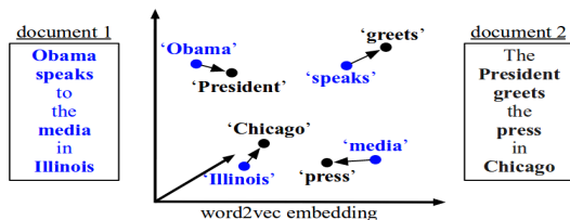
Figure: An illustration of the word mover's distance: All non-stop words (bold) of both documents are embedded into a word2vec space. The distance between two documents is the minimum cumulative distance that all words in document 1 need to travel to exactly match document 2
